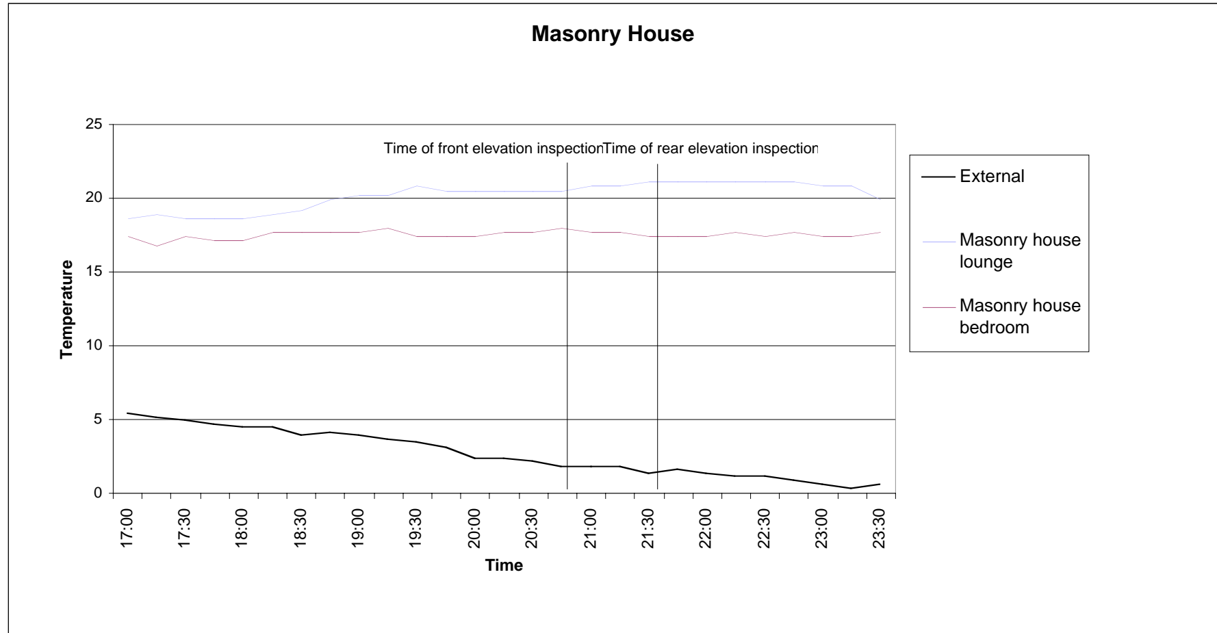
Figure 12 Temperature inside the masonry house on the evening of the thermographic survey
