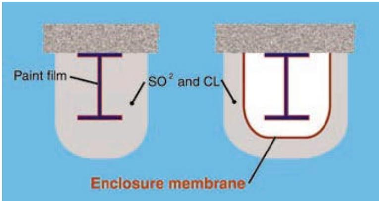
**Figure 3 : The Protection of Steelwork by Enclosure**
