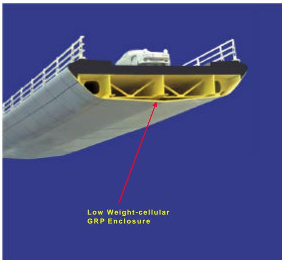
It is a structural floor suspended from the soffit of steel composite, plate girder [or concrete] bridges – see Figure 2. The floor and side membranes are formed in lightweight advanced composite material which encapsulate the structure.
