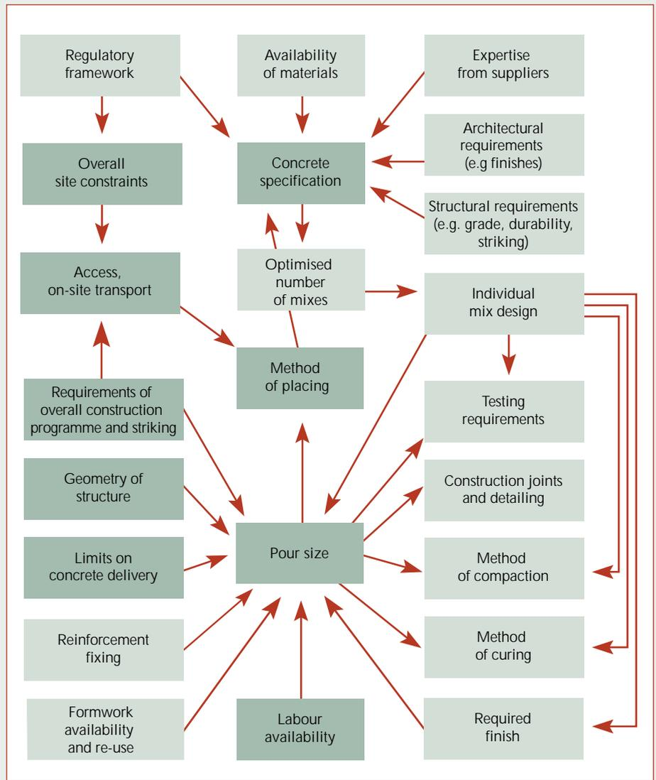
**Figure 2:** Issues and interactions affecting optimisation of concreting process for in-situ concrete frames. Key influences are highlighted
