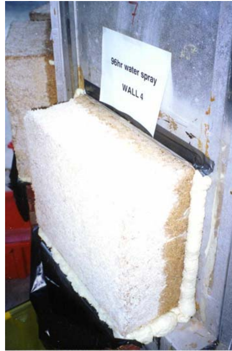
Figure 10. Water absorption depth after 96 hour water spray
