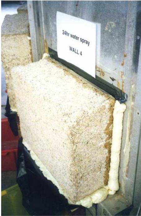
Figure 9. Water absorption depth after 24 hour water spray
