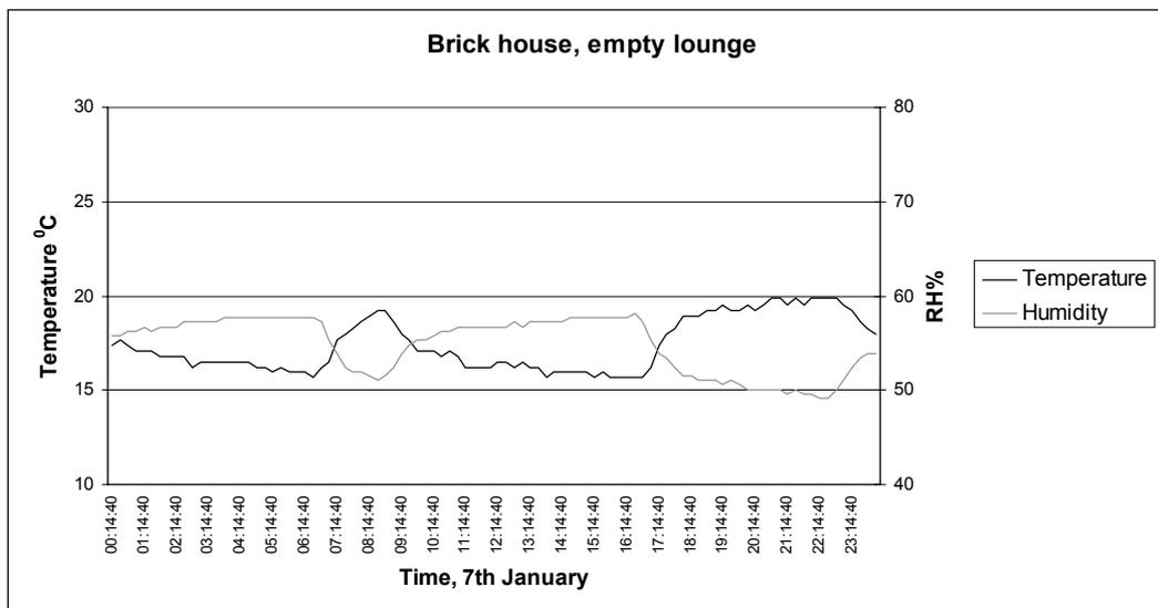
Figure 12. Comparison of the temperatures and humidities in the lounge of the traditional brick house and the hemp house – 7<sup>th</sup> January 2002
