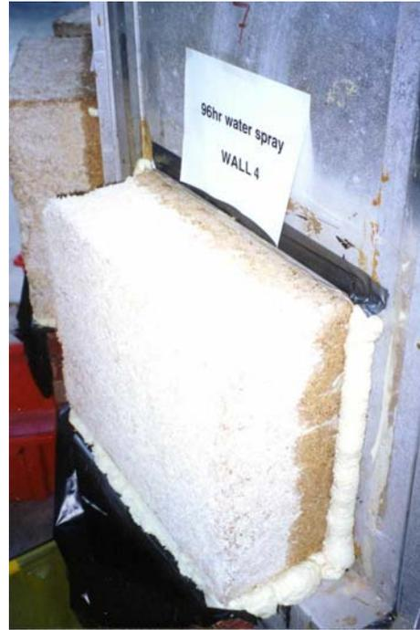
Figure 10. Water absorption depth after 96 hour water spray
