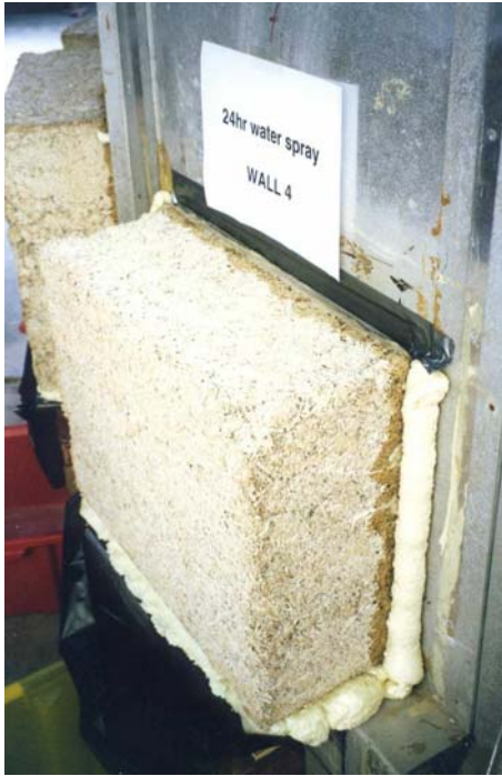
Figure 9. Water absorption depth after 24 hour water spray
