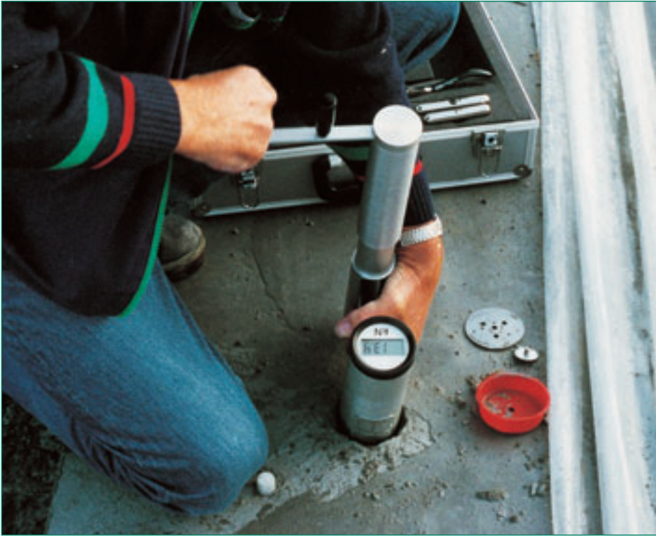
Figure 8: The Lok-test jack in position
